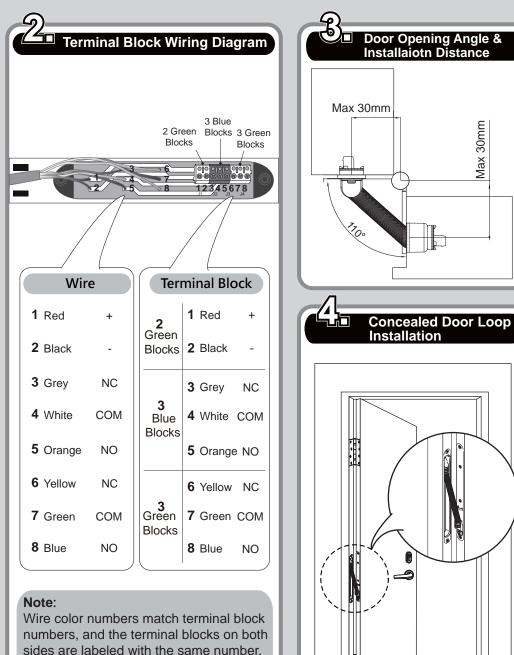
For each side, the Red wire 1 is connected to the terminal 1 of the Green Block, the Black wire 2 is connected to the terminal 2 of the Green Block, and so on.
