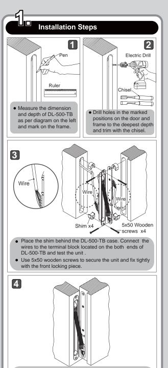
• Make sure the DL-500-TB is completely embedded into the door and frame.
